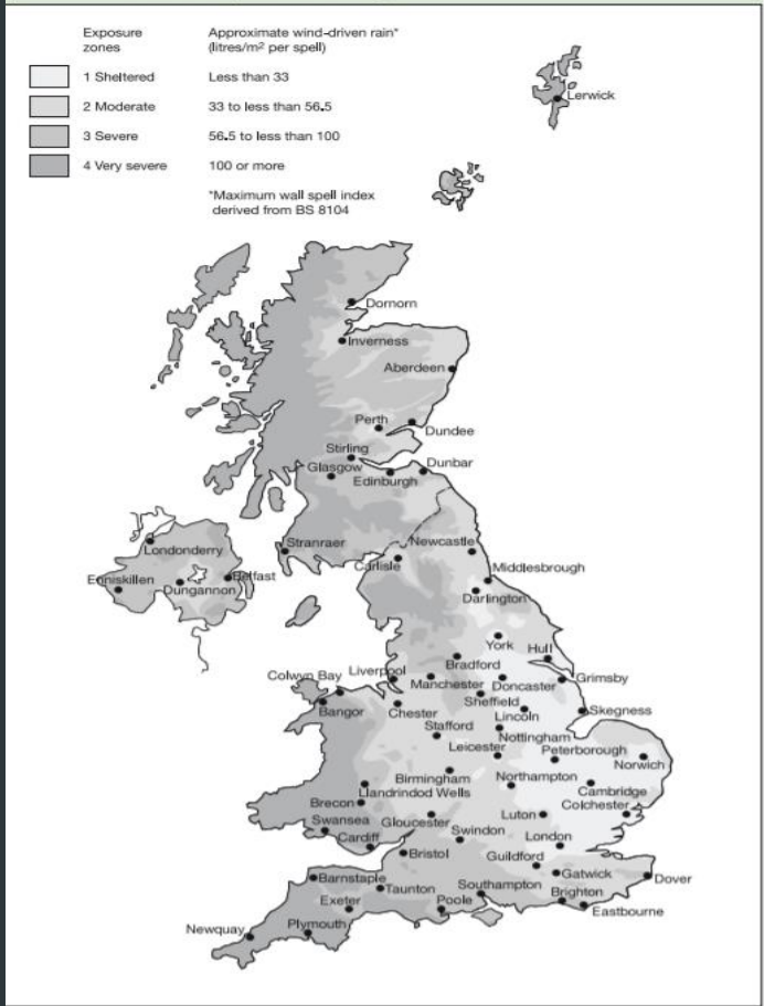
Diagram 12 UK zones for exposure to driving rain
