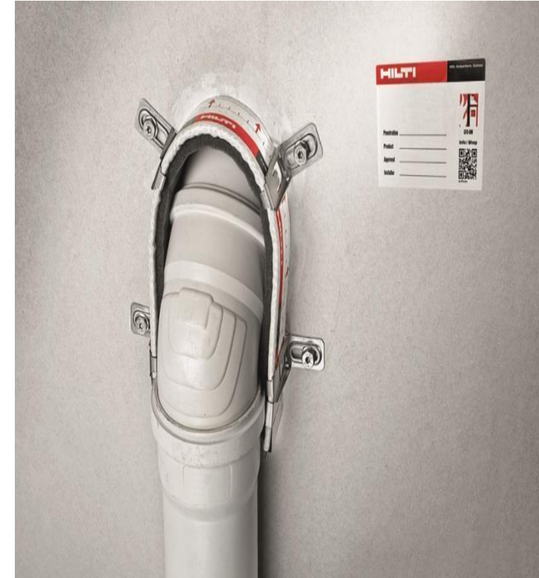
CFS-C EL Endless Collar Up to 120mins fire rating 16mm up to 160mm
